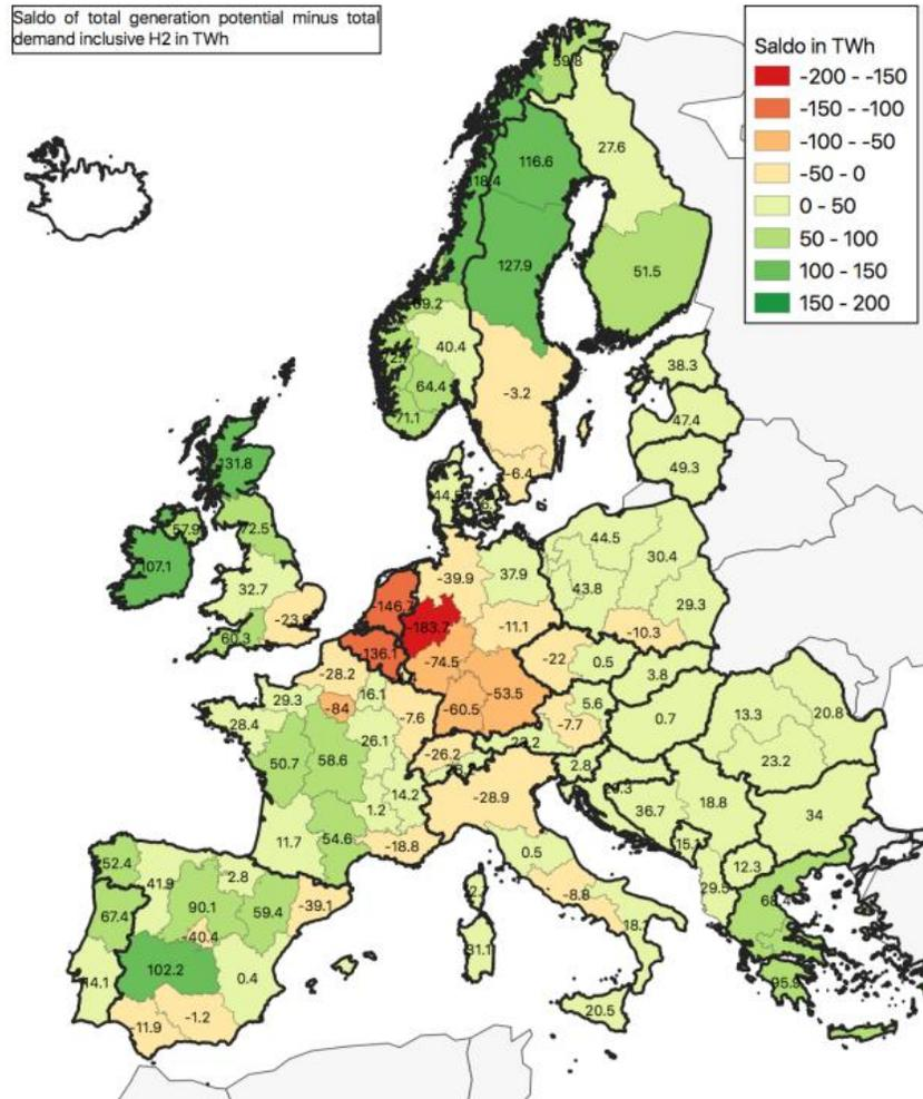
Figure 74: Balance of renewable generation potential and demand with electricity for hydrogen in Europe 2050.
