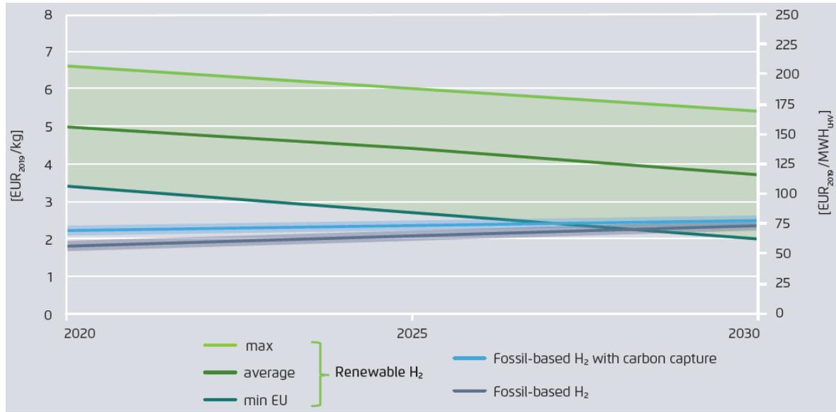
**Figure 67: Production cost of renewable H<sub>2</sub> compared to fossil-based H<sub>2</sub> with and without carbon capture. Source: Agora Energiewende and Guidehouse (2021, p. 14).**
