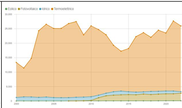
Figure 19: Development of electricity generation (GWh) by source (wind, PV, hydrogen power, thermo-electric) in Emilia-Romagna between 2000 and 2022. Source: [www.terna.it](http://www.terna.it)<sup>47</sup>
